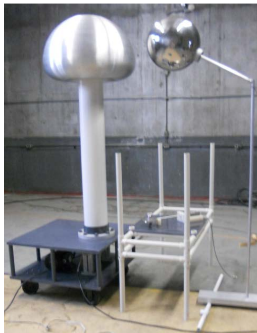
Figure 23. The initial D-dot sensor layout includes the electrode separation distance set at 5" with the sensor set 56" orthogonally below the center of the discharge arc.
