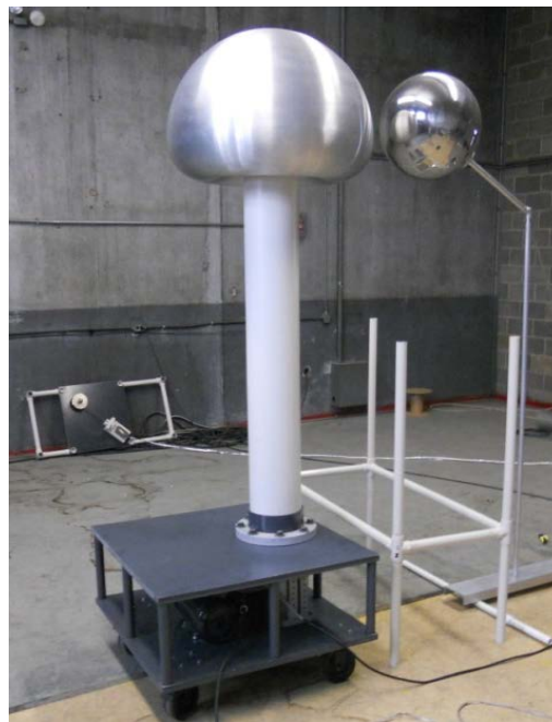
Figure 26. The layout is shown after applying shielding to the RG62 BNC transmission line and moving the D-dot sensor to 75" vertically below and 180" horizontally offset at the intersection of the laboratory wall and floor. The D-dot sensor area vector remains orthogonal to the discharging arc.
