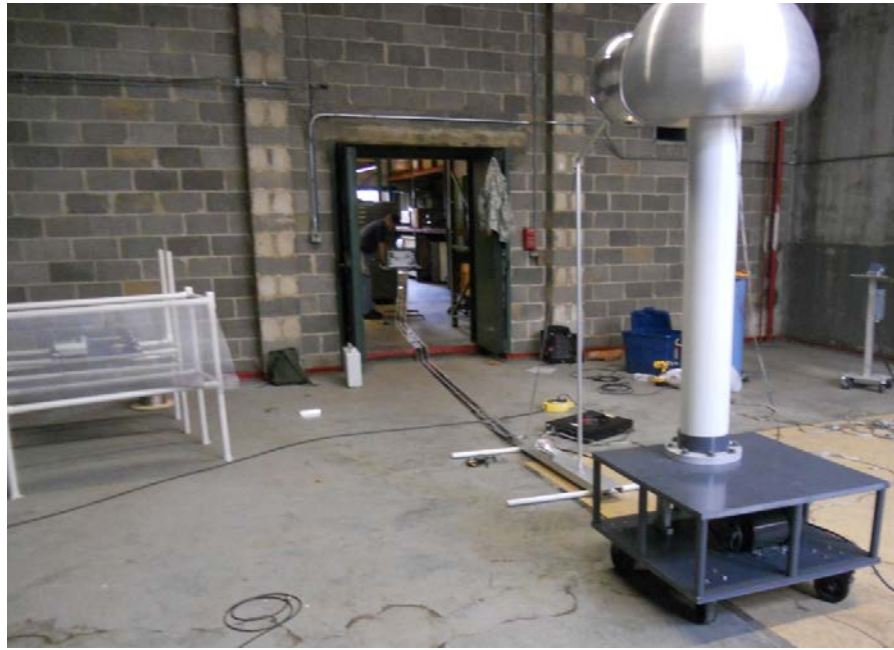
Figure 17. Layout with smooth aluminum tape ground loop connected to the ground strike globe. The CVR terminals were secured in series with the ground loop. The oscilloscope remained set just outside of the metal door threshold in line with the discharge arc axis approximately 25 ft from the center of the discharge arc.
