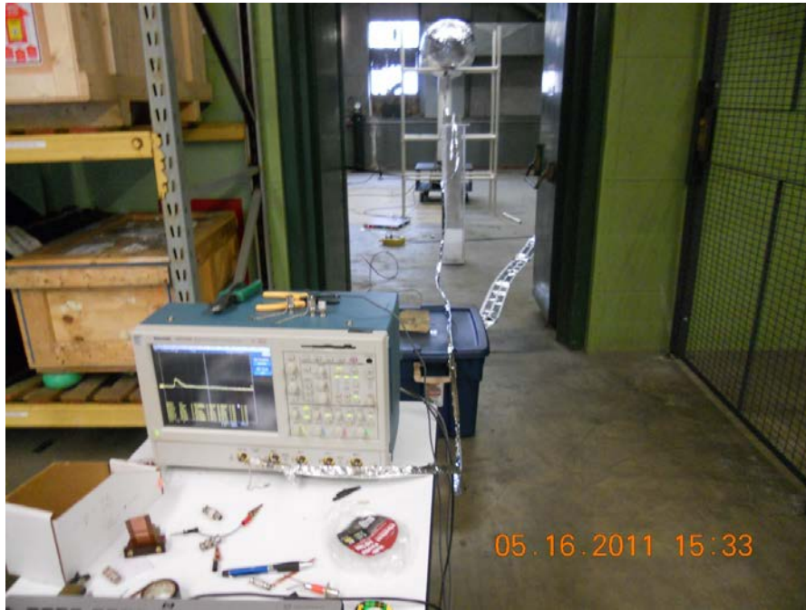
Figure 30. The CVR signal is transmitted on a 25 ft shielded RG62 BNC cable and displayed on an oscilloscope. The aluminum tape visible on the floor is disconnected and cast aside. This configuration was in use while collecting the Table 7 data.
