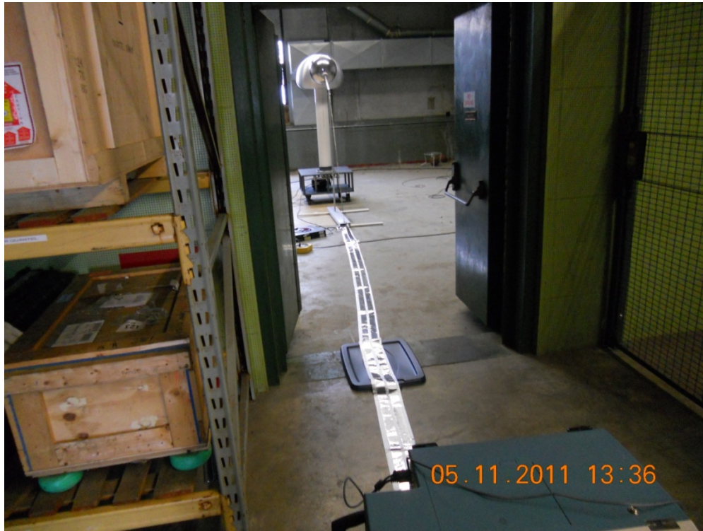
Figure 18. Laboratory layout with smooth aluminum tape ground loop connected to the ground strike globe which additionally highlights the extra insulation at the metal door threshold.
